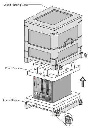
3. Release the clasp locks at the bottom, and lift the MGC+50 top cover.
